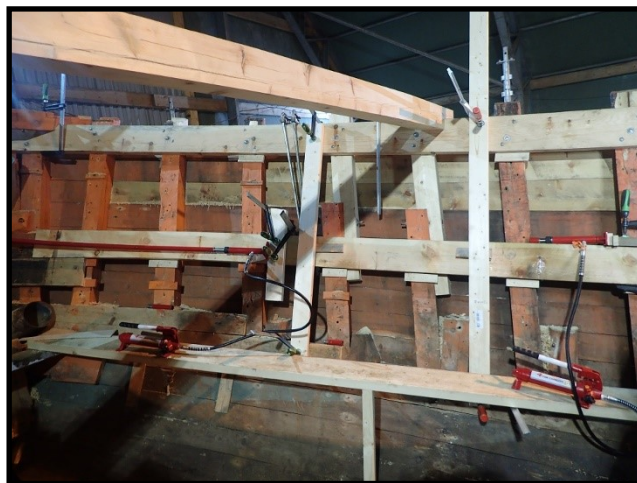
Vi bruke hydraulisk presse for montering.
